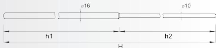
Tubular aluminium air termination rod consists of 2 parts: tube ø 16 mm and rod ø 10 mm, which are interconnected. To attach the wire to air termination rod use clamp art. C-041.
